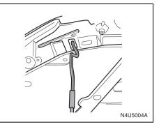
3) Lift the hood, release the hood prop from its retainer and place the hood prop into the slot in the hood.
